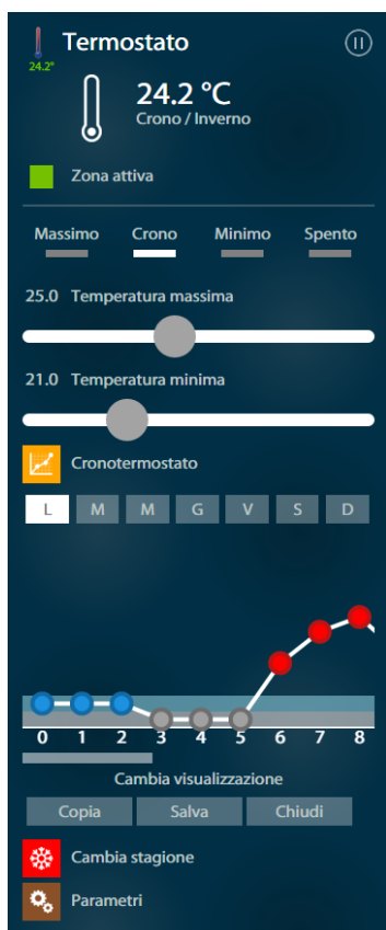
Figure 23. Full view of the state and the command of a temperature sensor in SideraHome
