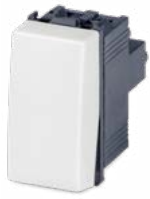
21000-AB ☼ 1P switch 16AX 250V~, with interchangeable key cover
