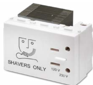
21190-AB Shaver socket with separation transformer 2P 127V~ and 230V~, 20 VA, 3 modules
