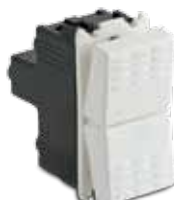
36022 Pulsador doble 1P/NA+1P/ NA+1P/ NC+1P/NC 16A 250V~, blanco
